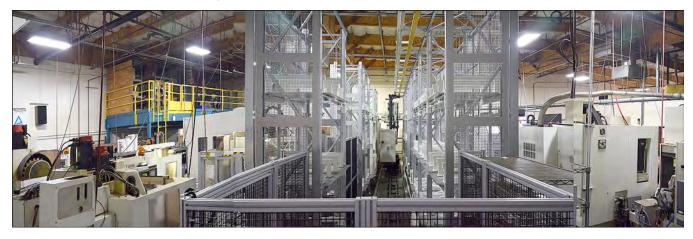
A view down a railway that transfers pallets to two five-axis CNC machining centers.
