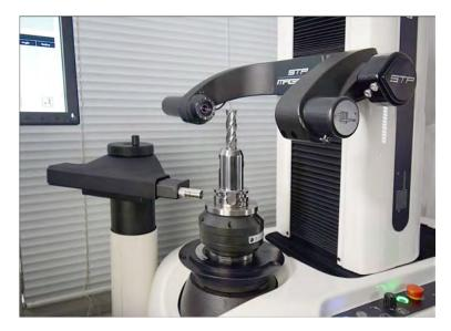
For Pacon, presetting tools offline helps avoid process delays and eliminate errors.
