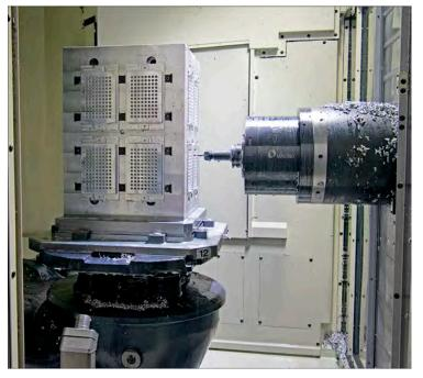
The five-axis Makinos accommodate both single-part setups and pallet-mounted tombstones that typify many horizontal machine setups.
